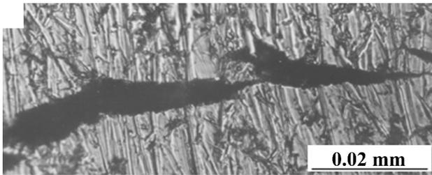
**Fig. 12.** Cleavage cracks in iridium single crystal having abraded working surface under tension.
